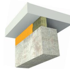
11/12. Single seal, exposed or unexposed side
