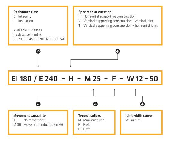
You may be asked the question: "Is your fire resistant joint seal able to accommodate movement?" Be careful! – It is not enough to use an elastic joint sealant with the required movement capability (e.g. according to ISO 11600 or ASTM C 920); because also specific fire resistance tests (e.g. according to EN 1366-4) must be performed under forced movement.
