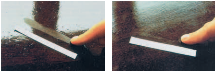
Fig. 10.1.1: Finger test of correct MRA application (left: too much MRA / right: good application of MRA)
