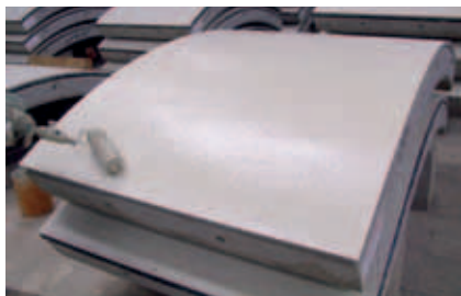
Fig. 8.4.4: Immediately following curing in a steam channel, the concrete surface of tunnel lining segments is coated with water-based epoxy emulsion that is absorbed even into the smallest pores, thereby generating a sealed, protective coating.
